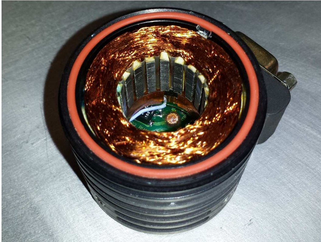
Figure 6. Inside the micro cooler motor stator. The blue wire at the center of the image was added to make contact with one of three hall sensors embedded in epoxy, in order to provide a readout of the rotor position.
