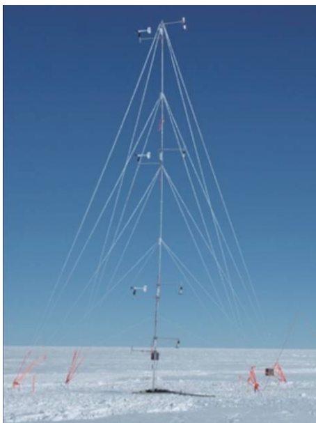
FIG. 1.—Kunlun Automated Weather Station (KL-AWS) installed at Dome A in January 2011. The propeller anemometers at 2 m, 4 m, 9 m, and 14.5 m are clearly visible. See the electronic edition of the PASP for a color version of this figure.
