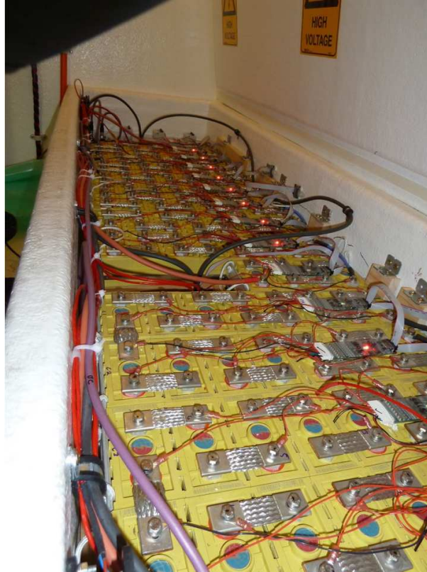
Figure 2. The PLATO-F LiFePO 4 battery pack, consisting of three parallel strings of 36 cells. The pack is in a separate polyurethane insulated box within the PLATO-F Instrument Module, to allow the cells to be kept warm with low power dissipation. The lid of the box is open in this photograph.
